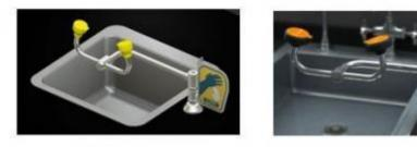
**Dual-Head Drench Hose -** A plumbed eyewash that is mounted on a countertop, usually next to a sink. The handle is attached to a flexible hose below the countertop. The eyewash can be used in place or pulled out for closer use. If used over a sink, it drains directly into the building plumbing through the sink drain.
