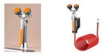
*Faucet-Mounted* - A plumbed eyewash that is mounted directly on a faucet. The eyewash drains directly into the building plumbing through the sink drain. Labs must contact EHS and Facilities to request installation of these units.
